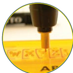
Standard - ink pen with lettering stencil.
